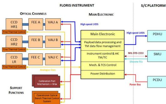
Figure 3-9: Electronics functional block diagram
