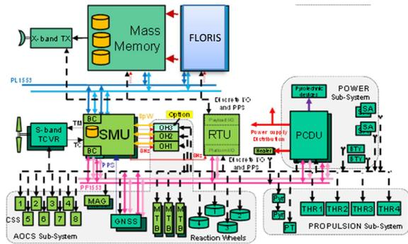
Figure 3-12: Satellite Avionics Architecture
