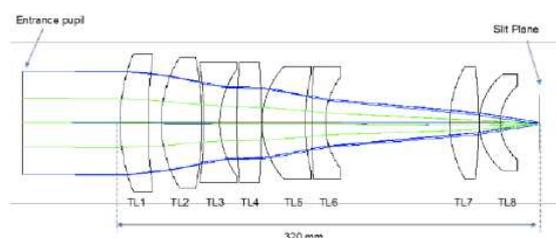
Figure 3-4: Telescope optical lay-out.
