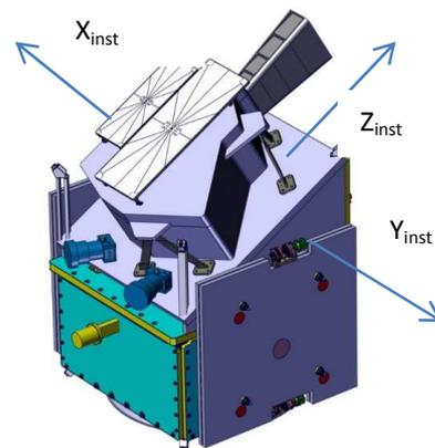
Figure 3-2: FLORIS Instrument on spacecraft (X<sub>inst</sub>=cold space, Y<sub>inst</sub>=speed direction, Z<sub>inst</sub>=Earth view)
