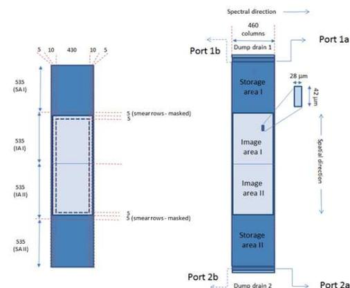
Figure 3-7: Detector configuration.
