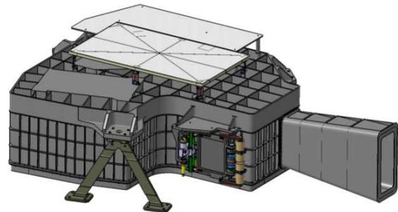
Figure 3-11: Mechanical layout (external view with baffle, radiators and solar port)
