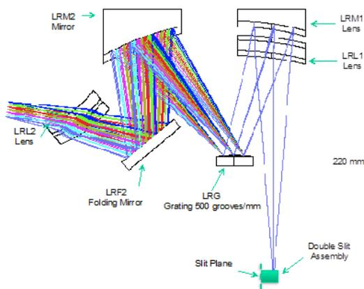
Figure 3-6: Low spectral resolution Spectrometer optical lay-out.
