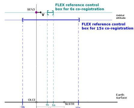
**Figure 2-1: Along track control boxes for 6 sec and 15 sec co-registration**
