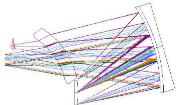
Figure 3-5: High Spectral Resolution Spectrometer optical lay-out.
